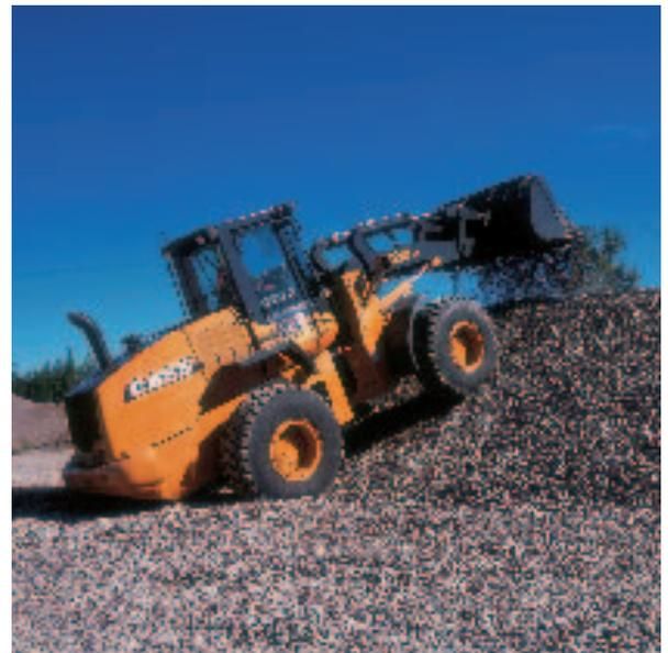
All specifications and dimensions given above are based on unit fitted with **20.5 R 25 XTLA Michelin** tyres, standard equipment. ROPS and FOPS cab, heavy counterweight, operator and full tanks. The dimensions and specifications comply with the ISO 8313, 5998, 7546 and pr EN 474-3.
