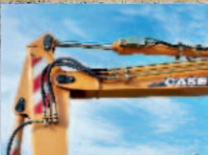
PATENTED ANTIDROP VALVES ON BOOM AND DIPPER CYLINDERS.
