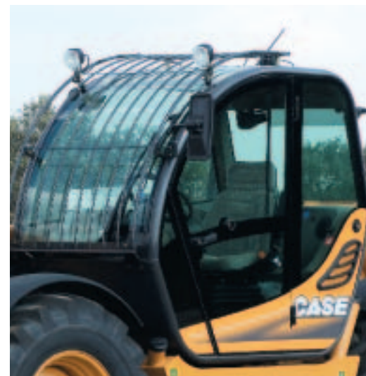
Cab door opens to 180° and secures at the fully open position. The door is constructed in two sections to enable the upper section to be opened independently.
