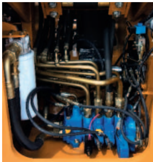
The "Load Sensing - Flow Sharing" hydraulic system grants totally independent movements. The rear-mounted control/valve is fully accessible without the need to move other components.
