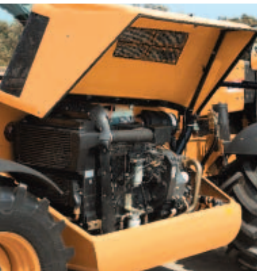
CNH TURBO 4.5 I engine The longitudinal engine mount ensures easy service.
